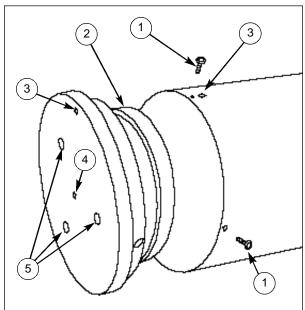
Fig. 3: Installing the Primary Mirror in the Optical Tube Assembly.
